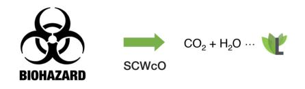
>85% heavy metals are recaptured for safe handling. Heavy metals are mainly detected in inert solid of the SCWcO effluent.
